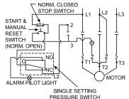
stops, and an alarm is sounded or light lights. (Note: Reverse NO and NC connections to pressure switch for same action on low pressure limit.)
